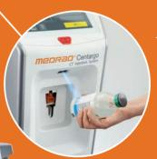
The bar code reader reduces manual data entry and provides easy traceability and access to contrast and injection details.\*
